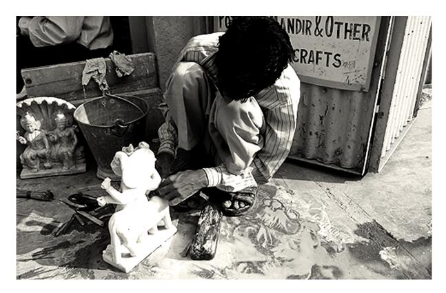
Figure 17 - Polishing takes place by rubbing different stones of various levels of smoothness
