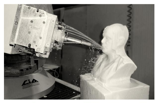
Figure 19 - Robotic Milling Process
