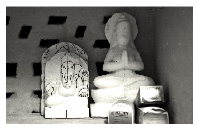
Figure 5 - The shape of the idol sketched onto the shaped marble blocks
