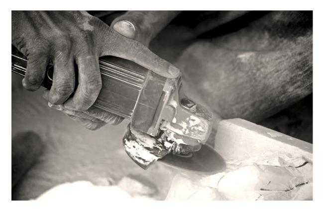
Figure 9 - Grinders used for the initial Shaping of the Raw Marble Blocks
