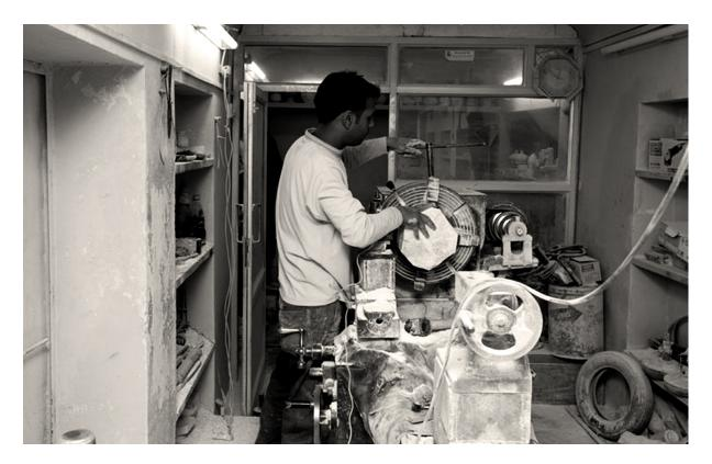
Figure 10 - Grinders used for the initial Shaping of the Raw Marble Blocks
