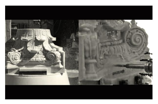
Figure 20 - Robotic Milling Process along with finished column base
