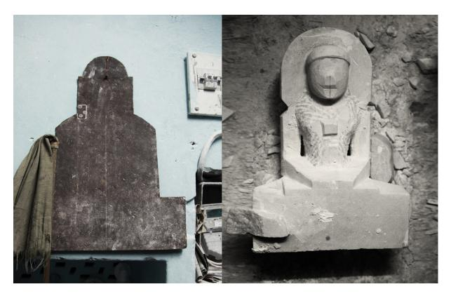
Figure 8 - Template used to size the Raw Marble Blocks when particular Idols are Mass-Produced
