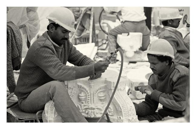
Figure 13 - Fine and sharp chisels are used to carve in the finer details and shapes of the carving
