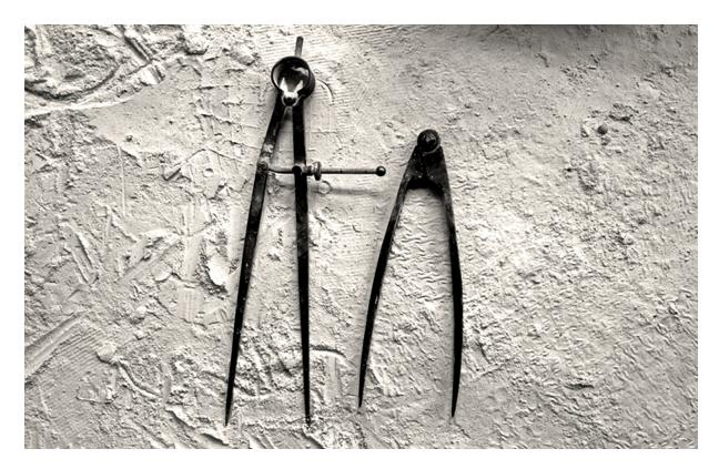
Figure 4 - The divider Prakaa - scaling tool
