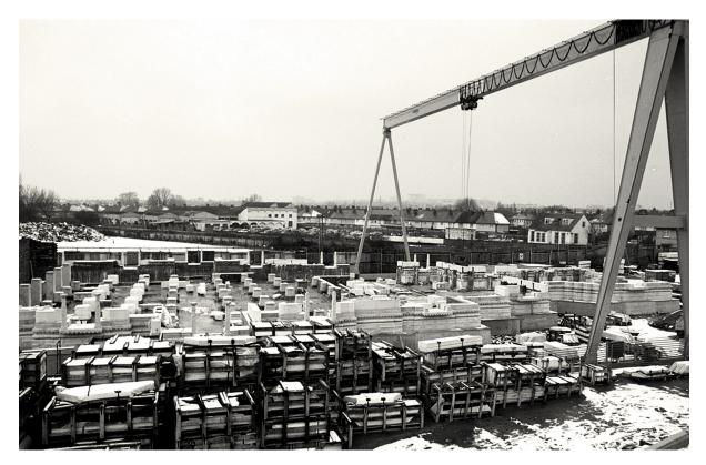
Figure 71 - Gantry cranes used for the assembly of the carved marble blocks
